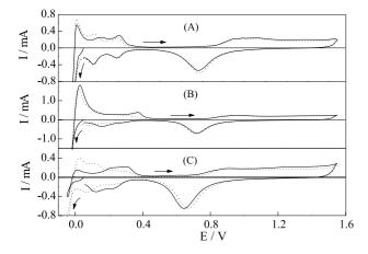
**Figure 2.** First-cycle voltammograms for Pt in 0.5 mol  $L^{-1} H_2SO_4$  (A), HClO<sub>4</sub> (B) and HF (C) at 0.2 V s<sup>-1</sup> and after the addition of: 1x10<sup>-5</sup> mol L<sup>-1</sup> (dotted lines) and 1x10<sup>-3</sup> mol L<sup>-1</sup> (full lines) ZnO. The cathodic potential incursion was extended up to -0.05 V, in the hydrogen evolution reaction region.
