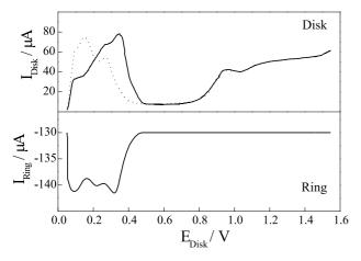
**Figure 3.** Linear sweep voltammograms for the disk electrode in the Pt/Pt rotating ring-disk system and the corresponding ring response in 0.5 mol L<sup>-1</sup> HF (dotted line) and after the addition of 10<sup>-3</sup> mol L<sup>-1</sup> ZnO (full line) to the electrolyte. Scan rate of 0.1 V s<sup>-1</sup>,  $E_{dep} = 300$  s,  $E_{ring} = -0.05$  V,  $\omega = 2.000$  rpm and collection factor = 0.195.
