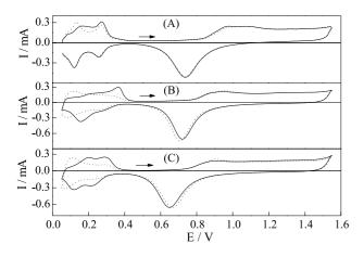
**Figure 1.** Steady-state profiles (dotted lines) for Pt in 0.5 mol  $L^{-1}$  H<sub>2</sub>SO<sub>4</sub> (A), HClO<sub>4</sub> (B) and HF (C) and first-cycle voltammograms at 0.2 V s<sup>-1</sup> after the addition of 1x10<sup>-3</sup> mol L<sup>-1</sup> ZnO (full lines). Prior to potential scanning, a delay time of 300 s at 0.05 V was imposed to the electrode in order to reach a maximum coverage with Zn<sub>ads</sub>.
