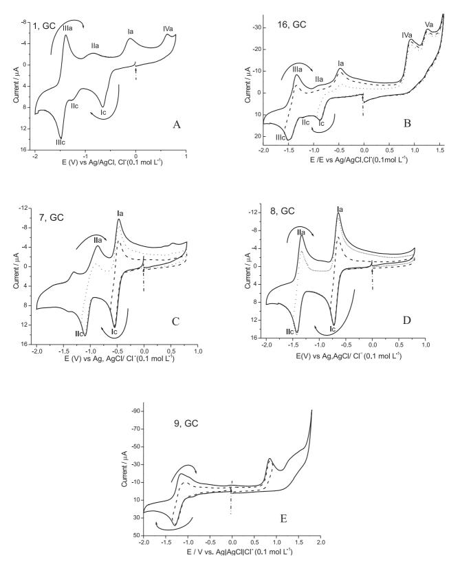
Figure 2. Cyclic voltammograms of the analysed compounds. E vs. Ag/AgCl, Cl<sup>-</sup>, 0.1 mol L<sup>-1</sup>. DMSO/TBAP or DMF/TBAP 0.1 mol L<sup>-1</sup> (**B**, **E**), glassy carbon electrode, n = 0.100 V s<sup>-1</sup>.
