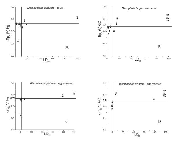
Figure 3. Plots of  $E_{plc}$  on Hg (A, C) and GC (B, D) electrodes *versus* molluscicidal activity (represented by LD<sub>90</sub> in ppm) against adult snails (A, B) and egg masses (C, D) of *Biomphalaria glabrata*.
