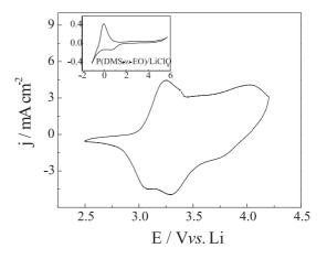
Figure 1. Steady state cyclic voltammogram of the PAnisilica|P(DMS-co-EO)|Li system, at 1 mV s<sup>-1</sup>. The inset shows the electrochemical stability window for the polymeric electrolyte at same scan rate.
