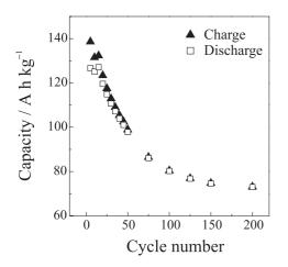
Figure 3. Dependence of the charge/discharge capacity on the number of cycles; current density of 1  $\mu$ A cm<sup>2</sup>.
