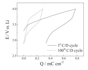
Figure 2. The first and 100<sup>th</sup> charge/discharge cycle; current density of 1  $\mu$ A cm<sup>-2</sup>.
