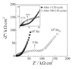
**Figure 4.** Nyquist diagram at the OCP potential (3.35 V) of the system after the first and  $100^{\text{th}}$  charge/discharge cycles. The inset shows the high frequency range.
