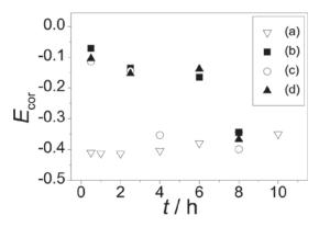
**Figure 11.**  $E_{\rm cor}$  values as a function of the immersion time, for immersion tests in aerated 0.4 mol L<sup>-1</sup> HCl for AISI-304 stainless-steel (a) non-colored samples and previously colored samples (with 200-250-nm oxide films) using the (b) alternating potential pulse, (c) triangular current scan and (d) chemical methods.
