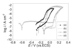
**Figure 8.** Typical potentiodynamic polarization curves (v = 0.2 mV s<sup>-1</sup>) obtained at 25 °C in dearated 0.62 mol L<sup>-1</sup> NaCl for AISI-304 stainless-steel (a) non-colored samples (as received) and previously colored samples (200-250-nm oxide films) using the (b) alternating potential pulse, (c) triangular current scan and (d) chemical methods.
