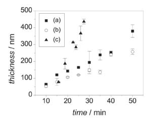
Figure 7. Thickness as a function of electrolysis/immersion time for oxide films grown on AISI-304 stainless steel using the (a) alternating potential pulse, (b) triangular current scan, and (c) chemical methods.
