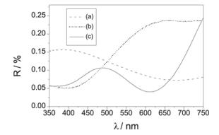
**Figure 3.** Reflectance spectra of stainless-steel samples colored using the triangular current scan method for different electrolysis times: (a) 15 min, (b) 30 min, and (c) 50 min.
