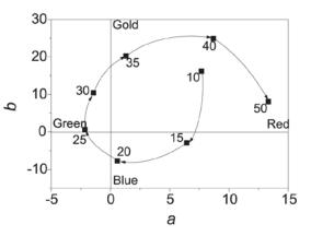
Figure 5. Chromatic coordinates of oxide films grown on AISI-304 stainless steel using the triangular current scan method for different electrolysis times (indicated alongside the points, in min).
