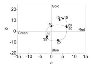
Figure 4. Chromatic coordinates of oxide films grown on AISI-304 stainless steel using the alternating potential pulse method for different electrolysis times (indicated alongside the points, in min).
