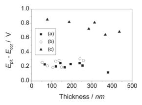
**Figure 9.**  $(E_{pit} - E_{cor})$  as a function of the thickness of the oxide films grown on AISI-304 stainless-steel samples using the (a) alternating potential pulse, (b) triangular current scan and (c) chemical methods.
