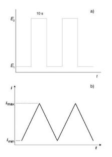
**Figure 1.** Diagrams illustrating the electrochemical methods used in the present study: (a) alternating potential pulses with  $E_1 = 0.35$  V,  $E_2 = 0.76$  V vs. Hg/Hg<sub>2</sub>SO<sub>4</sub>/5 mol L<sup>-1</sup> H<sub>2</sub>SO<sub>4</sub> and pulse width of 10 s; (b) triangular current scan with  $i_{max} = 2$  mA cm<sup>-2</sup>,  $i_{min} = -0.81$  mA cm<sup>-2</sup> and scan rate of 9 mA s<sup>-1</sup>.
