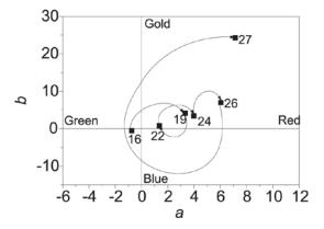
**Figure 6.** Chromatic coordinates of oxide films grown on AISI-304 stainless steel using the chemical method for different immersion times (indicated alongside the points, in min).
