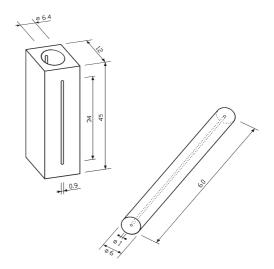
Figure 1. General view of the turbidimetric capillary glass cell and its support for the spectrophotometer. Dimensions expressed in mm.
