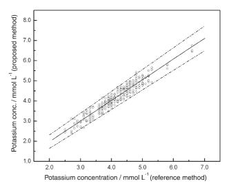
**Figure 4.** Comparison of the analytical results of the turbidimetric method with those of the selective electrode method, through a linear regression procedure (24). The dashed lines represent the confidence limits for 99% of confidence level.
