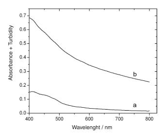
**Figure 2.** Visible spectra of solutions containing blood serum (400mL), sodium tetraborate buffer solution (400mL) and glycerin 10% aqueous solution (1.6 ml) plus 400mL of water (curve a) or 400mL of sodium tetraphenylborate 3% solution (curve b).
