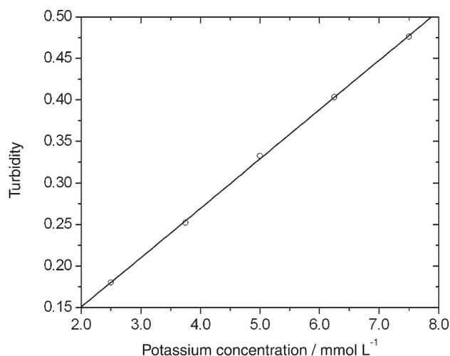
**Figure 3.** Calibration curve for the analysis of potassium in blood serum with the proposed turbidimetric method.
