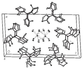
**Figure 3.** ORTEP3 view of KMt.4 $H_2O$  (1) showing the approximate hexagonal cavity that is formed by the packing of the anions along the b and the infinite chain of K( $H_2O$ )n units.
