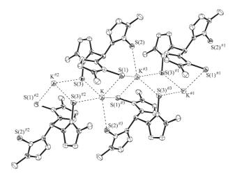
**Figure 5.** ORTEP3 view of the compound **2** showing in details the potassium coordenation environment. Displacement ellipsoids drawn at the 50% probability. (*Symmetry Codes:*  $^{#1} x+1$ , y, z;  $^{#2} -x$ , -y, -z;  $^{#3} -x+1$ , -y, -z).
