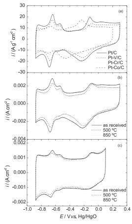
**Figure 7.** Cyclic voltammograms obtained for the Pt alloys in 1.0 mol  $L^{-1}$  KOH at 0.1 V s<sup>-1</sup>. (a) Comparison of the response of the different Pt alloys, (b) Pt-V/C thermally treated and (c) Pt-Cr/C thermally treated.
