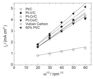
Figure 11. Levich plots for the ORR in the catalysts and for the Vulcan carbon in KOH 1.0 mol  $L^{-1}$  at 25 °C.
