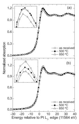
**Figure 3.** XANES spectra at the Pt  $L_3$  edge on thermally treated electrocatalysts in KOH 1.0 mol L<sup>-1</sup> at -0.7 V *vs.* Hg/HgO: (a) Pt-V/C and (b) Pt-Cr/C.
