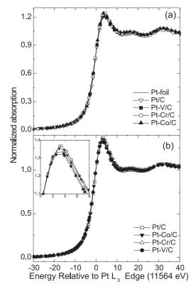
**Figure 2.** XANES spectra at the Pt  $L_3$  edge for the Pt/C, for as received Pt-M/C electrocatalysts and for a Pt-foil in KOH 1.0 mol L<sup>-1</sup>: (a) -0.7 V and (b) 0.2 V vs. Hg/HgO.
