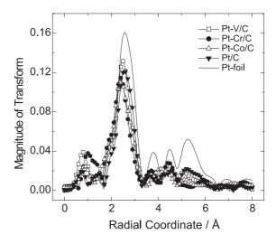
**Figure 5**. Fourier transform ( $k^3$  weighted) of the EXAFS oscillations for the as received Pt-M/C electrocatalyts at -0.7 V vs. Hg/HgO.
