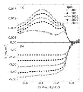
**Figure 8**. Rotating ring/disk results for the ORR in KOH 1.0 mol  $L^{-1}$  at 25 °C at several rotation speeds for the Pt-V/C electrocatalyst; (a) ring currents and (b) disk currents.
