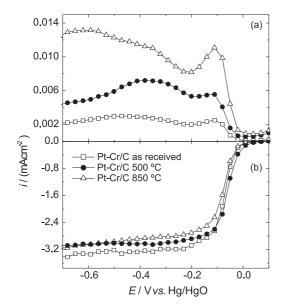
**Figure 10.** Rotating ring/disk results for the ORR in the Pt-Cr/C catalysts in KOH 1.0 mol  $L^{-1}$  at 25 °C and 1600 rpm: (a) ring currents and (b) disk currents.
