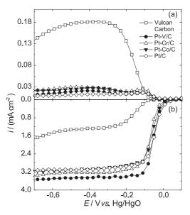
**Figure 9.** Rotating ring/disk results for the ORR in the |Pt/C and the as received Pt-M/C catalysts in KOH 1.0 mol  $L^{-1}$  at 25 °C and 1600 rpm: (a) ring currents and (b) disk currents.
