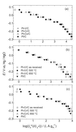
**Figure 12.** Mass-transport corrected Tafel plots for the ORR in the several catalysts in KOH 1.0 mol L<sup>-1</sup> at 25 °C.  $\varpi$  = 1600 rpm. (a) Comparison of the response of the different Pt-M/C alloys, (b) Pt-V/C thermally treated and (c) Pt-Cr/C thermally treated. Currents were normalized per mass of platinum in the catalyst layer.
