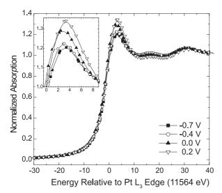
**Figure 1**. XANES spectra at the Pt  $L_3$  edge for the Pt/C electrocatalysts at different electrode potentials (*vs.* Hg/HgO) in KOH 1.0 mol L<sup>-1</sup>.
