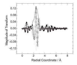
**Figure 6.** A first-shell fit of Pt EXAFS ( $k^3$  weighted) for Pt-V/C in r space: (solid line) experimental FT; (dotted line) experimental FT phase; fit of ( $\bullet$ ) FT amplitude and (O) phase.
