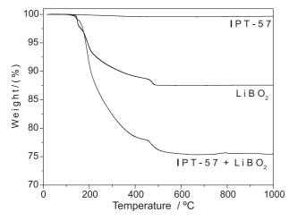
**Figure 3.** Thermogravimetric curves for LiBO<sub>2</sub> and for IPT-57 ground without modifier and with LiBO<sub>2</sub>.
