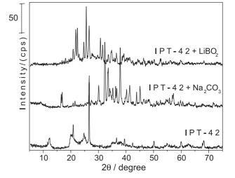
Figure 1. X-ray diffraction analysis of IPT-42 unmodified and modified with LiBO, or Na<sub>2</sub>CO<sub>3</sub>.
