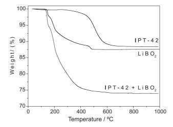
**Figure 2.** Thermogravimetric curves for  $LiBO_2$  and for IPT-42 ground without modifier and with  $LiBO_3$ .
