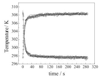
Figure 2. Time evolution of the sample temperature for two conditions: when the sample is illuminated by white light and when the light is turned off.
