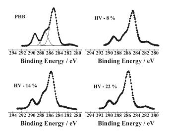
Figure 4. Photoemission spectra of the carbon 1s core level (C-1s) obtained for P(3HB) and P(3HB-co-3HV) with 8, 14 and 22 mol % of HV contents.
