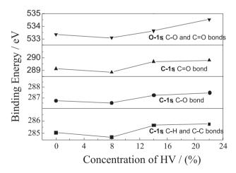
Figure 6. O-1s and C-1s binding energies dependence on the hydroxyvalerate content.
