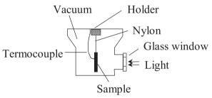
Figure 1. Scheme of the experimental arrangement used for specific thermal capacity determination.
