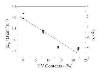
Figure 3. Dependence of specific thermal capacity,  $rc_p$  (square symbol), and glass transition temperature, Tg (star symbol), on the content of hydroxyvalerate.
