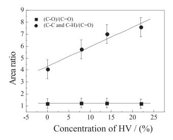
**Figure 5**. The HV content dependence for the ratio of the C-O species to C=O species (peaks area ratio obtained from Gauss-Lorentz curves) and for the ratio of the C-H and C-C species to C=O species.
