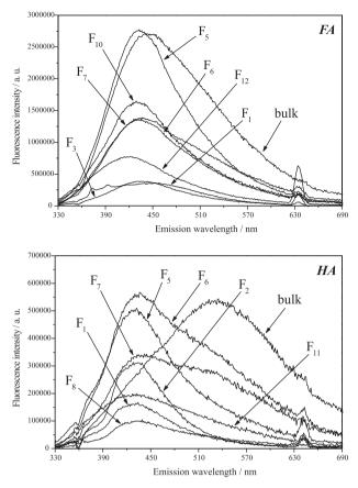
**Figure 7.** Single emission spectra ( $\lambda_{exc}$  = 320 nm) for the HPLC fractions. As in Fig. 6, the intensities were normalized, with the spectrum of the FA bulk sample being multiplied by 1.4 and that of the HA, divided by 1.6.
