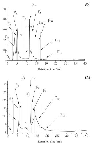
Figure 3. HPLC peaks for the estuarine HS obtained with a fluorescence detector ( $\lambda_{exc} = 320 \text{ nm} / \lambda_{emi} = 440 \text{ nm}$ ).
