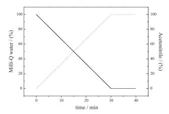
Figure 1. Gradient program for HS fractionation. (---) Milli-Q water, (----) acetonitrile.
