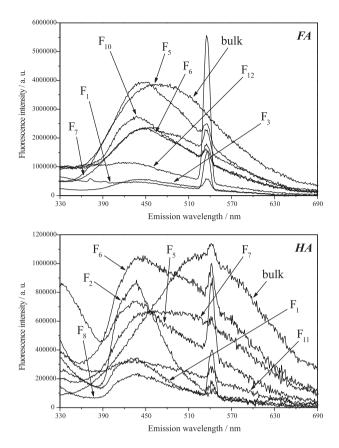
**Figure 6.** Single emission spectra ( $\lambda_{avc} = 270 \text{ nm}$ ) for the HPLC fractions. In order to facilitate comparisons, the intensities were normalized, with the spectrum of the FA bulk sample being multiplied by a factor of 1.2 and that of the HA, divided by a factor of 1.7.
