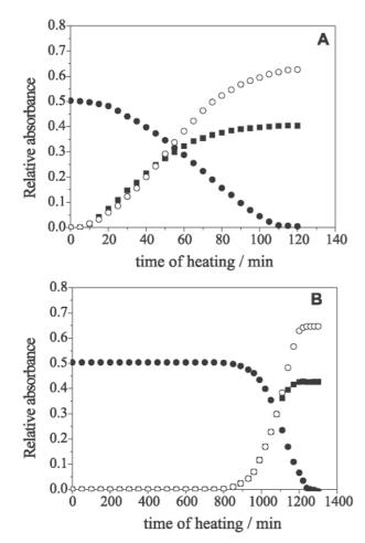
**Figure 3.** Kinetics of thermal-oxidation of polyisoprene film at 140 °C. (A) in absence of antioxidant; (B) in the presence of 5% of technical CNSL. Consumption of C=C ( $\bullet$ ) 835 cm<sup>-1</sup>; formation of C=O ( $\blacksquare$ ) 1720 cm<sup>-1</sup>; formation of OH/OOH ( $\bigcirc$ ) 3450 cm<sup>-1</sup>.
