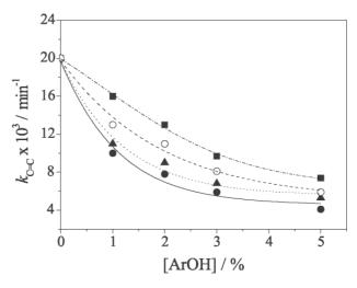
**Figure 7.** Effect of the antioxidant concentration on the apparent rate constant of C=C consumption during thermal oxidation of polyisoprene at 140 °C. Antioxidants: Hcardanol ( $\blacksquare$ ); Cardanol ( $\blacktriangle$ ); HAlkcardanol ( $\bigcirc$ ); Technical CNSL( $\odot$ ).
