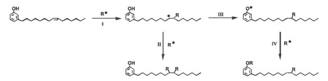
Figure 4. Suggested mechanism of cooperative action of hydroxyl and allyl groups in trapping rubber radicals (R<sup>\*</sup>).
