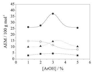
**Figure 6.** Effect of the antioxidant concentration on its effectiveness over thermal oxidation of polyisoprene at 140 °C. Antioxidants: Hcardanol ( $\blacksquare$ ); Cardanol ( $\blacktriangle$ ); HAlkcardanol ( $\bigcirc$ ); Technical CNSL( $\bigcirc$ ).
