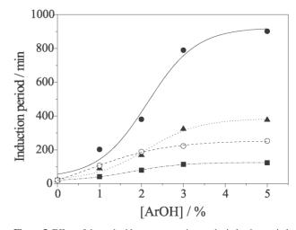
**Figure 5.** Effect of the antioxidant concentration on the induction period of the thermal oxidation of polyisoprene at 140 °C. Antioxidants: Hcardanol ( $\blacksquare$ ); Cardanol ( $\blacktriangle$ ); HAlkcardanol ( $\bigcirc$ ); Technical CNSL( $\odot$ ).
