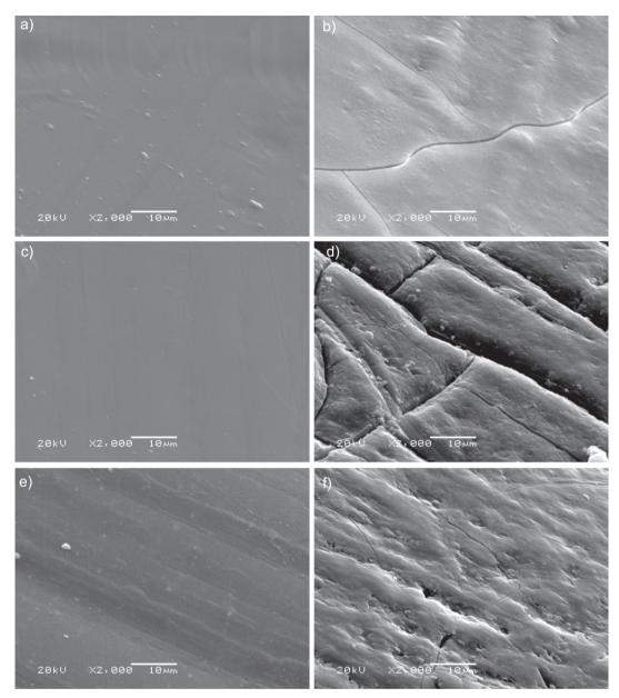
**Figure 7.** Scanning electron photomicrographs: polycarbonate (a) before and (b) after 3360 h of aging, polycarbonate containing anthraquinone dye (c) before and (d) after 3360 h of photochemical aging, polycarbonate containing bismuth vanadate (e) before and (f) after 3360 h of photochemical aging.
