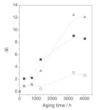
**Figure 4.** Color variation parameter ( $\Delta E$ ) as a function of aging time for: polycarbonate ( $\blacksquare$ ), polycarbonate containing anthraquinone dye ( $\bigcirc$ ), and polycarbonate containing bismuth vanadate pigment ( $\blacktriangle$ ).
