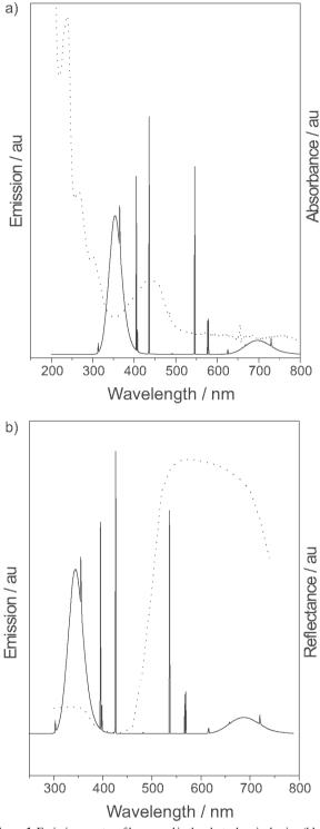
**Figure 1.** Emission spectra of lamp used in the photochemical aging (black line) and a) absorption spectrum of anthraquinone dye (dotted line), b) reflection spectrum of  $BiVO_4$  (dotted line).
