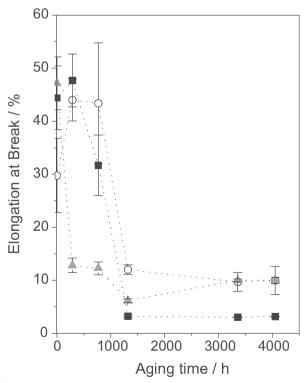
**Figure 2.** Elongation at break as a function of the aging time: polycarbonate ( $\blacksquare$ ), polycarbonate containing anthraquinone ( $\bigcirc$ ), and bismuth vanadate ( $\blacktriangle$ ).
