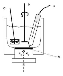
**Figure 1.** Scheme of the electrochemical cell used in the voltammetric and electrolytic experiments. (A) Working electrode (GDE or MGDE); (B) Reference electrode (Ag/AgCl, KCl sat.); (C) Counter electrode (platinum foil) and (D) Mechanical stirring. Volume of solution: 250 mL.
