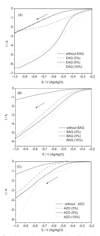
**Figure 2.** Linear voltammetry (LV) of GDEs modified by: (A) 2-ethylanthraquinone (EAQ); (B) 2-terc-butylanthraquinone (BAQ); and (C) azobenzene (AZO). Oxygen-purged supporting electrolyte, pressure of 0.16 Bar. Supporting electrolyte 0.1 mol L<sup>-1</sup>  $\rm H_2SO_4$ ,  $\rm v = 20~mV~s^{-1}$ ,  $\rm T = 20~^{\circ}C$ , mechanical stirring.
