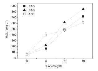
**Figure 8.** H<sub>2</sub>O<sub>2</sub> electrogeneration after 1 hour of electrolysis at -0.6 V vs. Ag/AgCl as function of the concentration of each catalyst used as GDE modifier.
