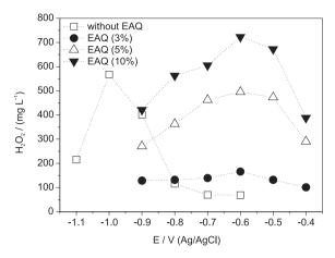
**Figure 5.**  $H_2O_2$  production after 1 hour of electrolysis with EAQ, as function of applied potential. Supporting electrolyte 0.1 mol  $L^{-1}H_2SO_4$  plus 0.1 mol  $L^{-1}K_3SO_4$ , v = 20 mV  $s^{-1}$ , T = 20 °C,  $O_2$ , flow (P = 0.16 bar).
