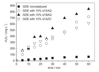
**Figure 4.**  $H_2O_2$  production as function of electrolysis time for GDE modified by 10% of catalysts. Supporting electrolyte 0.1 mol  $L^1$   $H_2SO_4$  plus 0.1 mol  $L^1$   $K_3SO_4$ , v = 20 mV  $s^{-1}$ , T = 20 °C,  $O_2$  flow (P = 0.16 bar).
