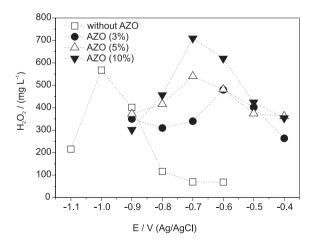
**Figure 7.**  $H_2O_2$  production after 1 hour of electrolysis with AZO, as function of applied potential. Supporting electrolyte 0.1 mol  $L^{-1}$   $H_2SO_4$  plus 0.1 mol  $L^{-1}$   $K_2SO_4$ , v=20 mV  $s^{-1}$ , T=20 °C,  $O_2$  flow (P=0.16 bar).
