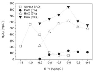
**Figure 6.**  $H_2O_2$  production after 1 hour of electrolysis with BAQ, as function of applied potential. Supporting electrolyte 0.1 mol L<sup>-1</sup>  $H_2SO_4$  plus 0.1 mol L<sup>-1</sup>  $K_4SO_4$ , v = 20 mV s<sup>-1</sup>, T = 20 °C,  $O_2$ , flow (P = 0.16 bar).
