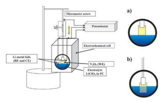
**Figure 1.** Cell showing the new electrochemical setup, implemented to be able to maximize, or to minimize the contact between sample and electrolyte. In the two insets: according to micrometer screw position we can have a) only film edge exposed, or b) most of film surface exposed to the electrolyte.
