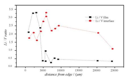
Figure 7. Evolution of Li/V ratios from the intercalated edge (only part in contact with solution) to top of the sample.
