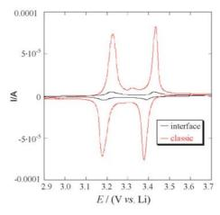
**Figure 3.** SSCV at 0.5 mV s<sup>-1</sup> taken either with most of film surface exposed ("classic"), or with only the film edge exposed to the electrolyte ("interface").
