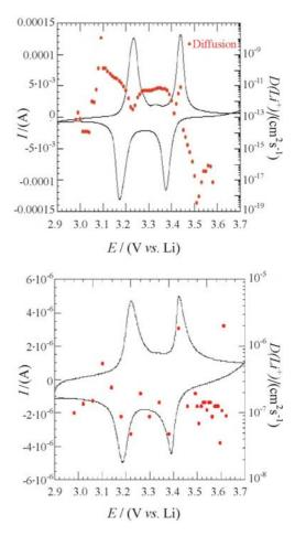
**Figure 4.** SSCV at 0.5 mV s<sup>-1</sup> (solid line) and Li diffusion coefficient deduced from PITT (red dots) for a "classic" insertion experiment (upper graph). The same exposing to the electrolyte only the edge of the film ("interface" experiment, lower graph).
