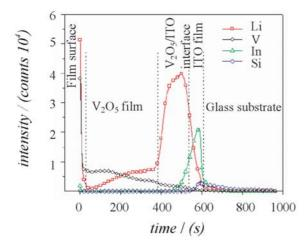
Figure 5. Typical SIMS depth profile of  $\mathrm{V_2O_5}$  thin film intercalated with Li ions
