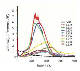
**Figure 6.** SIMS depth-profiles from edge intercalated sample. The vanadium profile from  $V_2O_5$  is indicated - all other profiles are of Li from the first 9 points indicated by square symbols on Figure 2.
