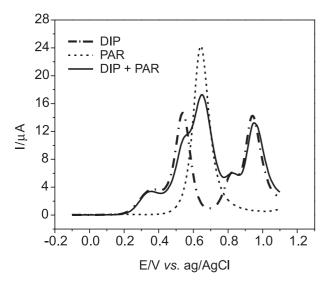
**Figure 4.** Differential pulse voltammograms of paracetamol (PAR), dypirone (DIP) and a mixture of DIP and PAR (both in concentration of  $1 \times 10^{-3}$  mol L<sup>-1</sup>) obtained using a carbon paste electrode. Supporting electrolyte: NaCl 0.5 mol L<sup>-1</sup> (pH 6.0). Potential range of: -0.1 V to 1.1 V vs. Ag/AgCl, scan rate: 25 mV s<sup>-1</sup>, time pulse: 100 ms, sensibility: 100  $\mu$ A V<sup>-1</sup>.
