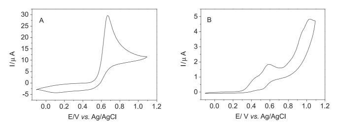
Figure 3. Cyclic voltammograms of (A) paracetamol and (B) dypirone, (concentration of  $1.0 \times 10^{-3}$  mol L<sup>-1</sup>) obtained using a carbon paste electrode in NaCl 0.5 mol L<sup>-1</sup> (pH 6.0). Potential range of: -0.1 V to 1.1 V vs. Ag/AgCl.
