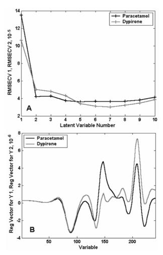
**Figure 5.** (A) RMSECV for PLSR model to determination of DIP and PAR; (B) Regression Coefficient with four Latent Variables in PLSR model.
