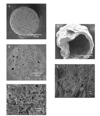
**Figure 1.** Scanning electron micrographs of PHB/PXC microparticles obtained through the procedure denoted as M7: (A) complete microparticle (B) inner part incorporated in a glycerol polyglycidyl ether resin, and (C) surface with higher magnification. Microparticles obtained using the conditions of M2: (D) fractured microparticle, and (E) surface.
