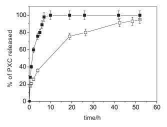
**Figure 4.** Release profiles of PXC from microparticles obtained under: ( $\blacksquare$ ) M2 and ( $\square$ ) M7 conditions, in phosphate buffer pH 7.4.
