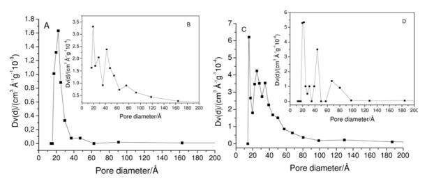
Figure 5. Pore diameter distribution curves, based on the BJH method: (A) M2 microparticles; (B) M2 microparticles after 8 h in phosphate buffer pH 7.4; (C) microparticles M7; (D) microparticles after 50 h in phosphate buffer pH 7.4.
