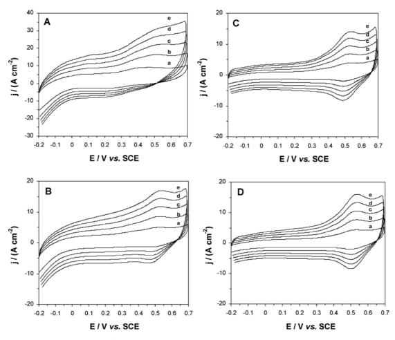
Figure 2. CV responses in aqueous 0.1 mol  $L^{-1}$  KF at 298 K of the four types of electrode: (A) Au/SAM/PG1-Fc, (B) Au/SAM/PG2-Fc, (C) Au/SAM/PG3-Fc, and (D) Au/SAM/PG4-Fc at (a) 0.1, (b) 0.2, (c) 0.3, (d) 0.4, and (e) 0.5 V s<sup>-1</sup>.
