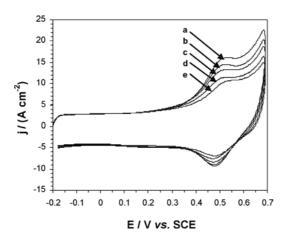
**Figure 3.** CV responses at dE/dt= 0.5 V s<sup>-1</sup> in 0.1 mol L<sup>-1</sup> KF at 298 K at various concentrations of βCD for the modified electrodes Au/SAM/PG4-Fc after the introduction of (a) 0, (b) 0.001, (c) 0.1, (d) 0.5, and (e)  $1 \times 10^{-3}$  mol L<sup>-1</sup> βCD. A similar trend was observed for the curves obtained for the systems Au/SAM/PG2-Fc and Au/SAM/PG3-Fc.
