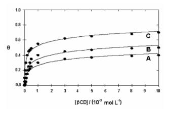
Figure 4. Adsorption isotherms of βCD from 0.1 mol L<sup>1</sup> KF at 298 K onto dendrimer-tethered ferrocene on the modified gold electrodes: (A) Au/SAM/PG2-Fc, (B) Au/SAM/PG3-Fc, and (C) Au/SAM/PG4-Fc. Experimental points derived from Figure 3 (•) were fitted to the Frumkin isotherm model, Equation 9 (—).
