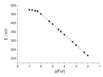
**Figure 2.** Calibration graph for the Fur-sensitive electrode with composition of 50% (Graphite, m/m). Experimental conditions: pH = 8.5,  $\mu = 0.500$  mol L<sup>-1</sup> adjusted with NaNO<sub>4</sub>, T = 25 °C.
