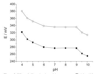
Figure 3. Effect of pH on the electrode's response at: ( $\blacksquare$ )  $1.0 \times 10^{-3}$  mol L<sup>-1</sup> Fur, ( $\bigcirc$ )  $1.0 \times 10^{-4}$  mol L<sup>-1</sup> Fur ;  $\mu = 0.500$  mol L<sup>-1</sup> adjusted with NaNO<sub>3</sub>, T = 25 °C.
