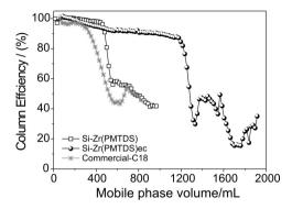
**Figure 5.** Variation of the column efficiencies of non-endcapped and endcapped SiZr(PMTDS) and of a commercial chemically-bonded  $C_{18}$  stationary phase. Mobile phase: MeOH:0.050 mol  $L^{-1}$   $K_2CO_3$  at pH 10; flow rate: 1.0 mL min<sup>-1</sup>; temperature: 50 °C; test probe: acenaphthene.
