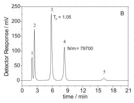
**Figure 4.** Separation of a test mixture on 60 mm  $\times$  3.9 mm columns containing (A) non-endcapped and (B) endcapped SiZr(PMTDS). Mobile phase: MeOH:H<sub>2</sub>O (70:30, v/v); flow rate: 0.3 mL min<sup>-1</sup>; injection volume: 5  $\mu$ L; detection: UV at 254 nm; temperature: 40 °C. Peak identifications: (1) uracil, (2) phenol, (3) *N*,*N*-dimethylaniline, (4) naphthalene and (5) acenaphthene.
