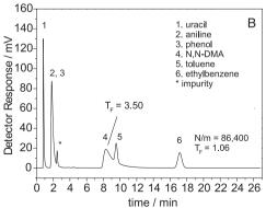
**Figure 1.** Chromatograms obtained on 60 mm  $\times$  3.9 mm columns containing (A) SiZrC<sub>18</sub>-carb phase or (B) SiZrC<sub>18</sub>-phase. Chromatographic conditions: MeOH:H<sub>2</sub>O (55:45, v/v); flow rate: 0.6 mL min<sup>-1</sup>; injection volume: 5  $\mu$ L; detection: UV at 254 nm. Peak identifications: (1) uracil, (2) aniline, (3) phenol, (4) *N*,*N*-dimethylaniline, (5) toluene, (6) ethylbenzene.
