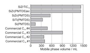
**Figure 8.** Hydrolytic stability of laboratory-made stationary phases and several different commercial stationary phases. Mobile phase volume (calculated from mobile phase retention determined using uracil) that causes a 50% decrease in the column efficiency measured with acenaphthene while passing MeOH:0.050 mol L<sup>-1</sup> K<sub>2</sub>CO<sub>3</sub>/KHCO<sub>3</sub> (nominally pH 10) mobile phase at 50 °C.
