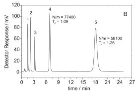
**Figure 2.** (A) Separation of (1) codeine, (2) prilocaine, (3) N,N-dimethylaniline, (4) naphthalene and (5) and amitriptyline on a 60 mm  $\times$  3.9 mm SiZrC $_{18}$ -carb column at 0.6 mL min $^{-1}$ , using MeOH:0.050 mol L $^{-1}$  hexamethylenimine (HMI) buffer (60:40, v/v) at 40 °C. (B) Same separation after 100 consecutive injections.
