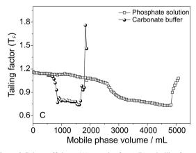
**Figure 6.** Column efficiency (A), retention factor (B) and tailing factor (C), calculated for acenaphthene, during stability tests on 60 mm  $\times$  3.9 mm columns packed with a commercial  $C_{18}$  phase. Mobile phase: (70:30, v/v) MeOH:0.050 mol  $L^{-1}$   $K_2HPO_4$  solution or  $K_2CO_3/KHCO_3$  buffer at pH 10.0; flow rate: 0.6 mL min $^{-1}$ ; temperature: 50 °C.
