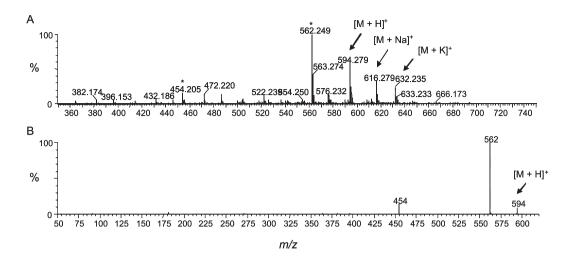
Figure 3. A: ESI-MS of product 19; B: ESI-MS/MS of the protonated molecules of 19. Ions marked by an asterisk are fragments due to CH<sub>3</sub>OH and PhCH<sub>3</sub>OH loss that arise likely from in-source collision-induced dissociation.
