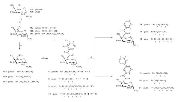
**Scheme 1.** Reagents and conditions: (a)  $Bu_4NBr$ , 50% m/v aqueous NaOH,  $CH_2Cl_2$  or ethyl ether, allyl bromide or 5-bromo-1-pentene, rt; (b) LiAlH4, THF, rt; (c) 3- or 2-iodobenzoyl chloride (2 equivalents), 10% m/v aqueous NaOH,  $CH_2Cl_2$ , ice bath; (d)  $Bu_3SnH$  (1.5 equivalents), AIBN (catalytic amount), benzene,  $N_2$ , reflux.
