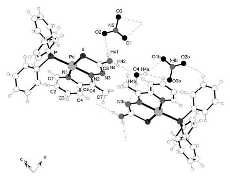
Figure S1. View of the crystal structure of [Pd(aptsc)(PPh<sub>3</sub>)](NO<sub>3</sub>)·H<sub>2</sub>O (1) toward the direction [001], showing the hydrogen bonds as dashed lines.
