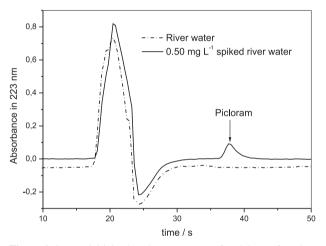
**Figure 4.** Sequential injection chromatograms of a picloram free river water superposed to a chromatogram of the same sample spiked with 0.50 mg  $L^{-1}$  of picloram, exhibiting the absence of interference peaks in the retention time of the analyte. The large and high peak at 20.5 s is assigned to unretained substances with strong absorption of UV radiation.
