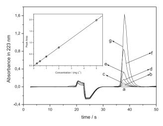
**Figure 2.** Sequential Injection Chromatograms for calibration of the SIC system obtained by injecting 100  $\mu$ L of standard at flow rate of 30  $\mu$ L s<sup>-1</sup> in a mobile phase composed by 20:80 ACN: 5.0 mmol L<sup>-1</sup> H<sub>3</sub>PO<sub>4</sub> Picloram concentrations of the calibration solutions were: (a) blank, (b) 0.25, (c) 0.50, (d) 1.0, (e) 2.0, (f) 5.0 e (g) 10 mg L<sup>-1</sup>. The inset shows the linear correlation between peak area and picloram concentration.
