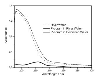
**Figure 3.** Absorption spectrum of a 0.50 mg  $L^{-1}$  picloram solution in deionized water superposed to the spectra of a river water sample and river water spiked with 0.50 mg  $L^{-1}$  of picloram.
