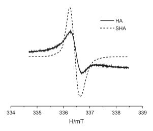
Figure 2. EPR spectrum of the humic acid (HA) sample extracted from soil, and of the sample synthesized from *para*-benzoquinone (SHA without metals), showing the free radical signal.
