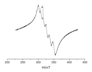
Figure 5. EPR spectrum of the SHA sample with manganese.
