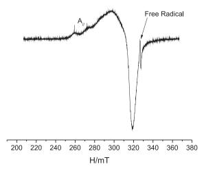
Figure 3. EPR spectrum of the SHA sample complexed with copper: T = 90 K and A<sub>u</sub> is hyperfine coupling.
