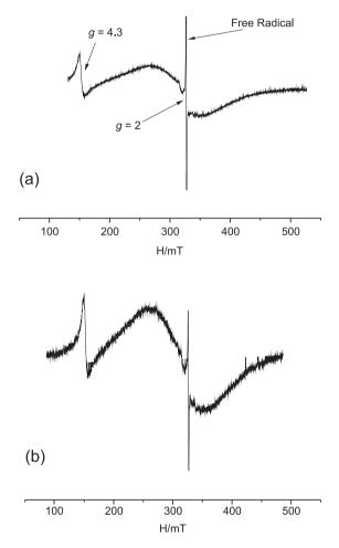
Figure 4. EPR spectrum of (a) the HA sample extracted from soil, and (b) SHA with iron.
