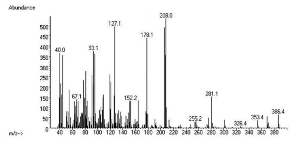
$\textbf{Figure S6.} \ \, \textbf{GC-MS} \ \, (\textbf{TIC}) \ \, \textbf{chromatogram} \ \, (\textbf{abscissa: scan number, ordinate: relative response of MS detector)} \ \, \textbf{and AMS profile (abscissa: } \textit{m/z} \ \, \textbf{value, ordinate: response of MS detector)} \ \, \textbf{of model complex mixture M4.}$
