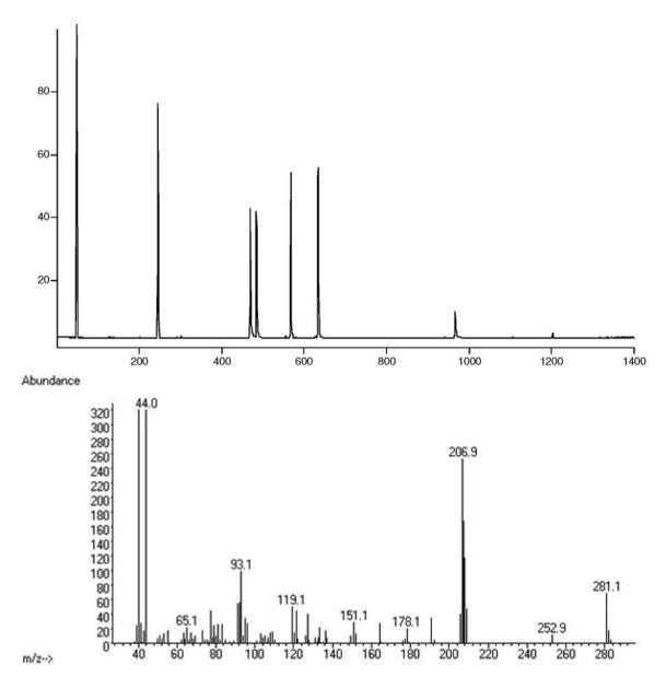
**Figure S3.** GC-MS (TIC) chromatogram (abscissa: scan number, ordinate: relative response of MS detector) and AMS profile (abscissa: m/z value, ordinate: response of MS detector) of model complex mixture M1.
