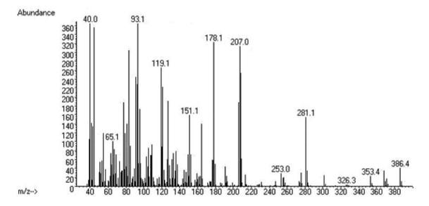
$\textbf{Figure S8.} \ \, \textbf{GC-MS} \ \, (\textbf{TIC}) \ \, \textbf{chromatogram} \ \, (\textbf{abscissa: scan number, ordinate: relative response of MS detector)} \ \, \textbf{and AMS profile (abscissa: } \textit{m/z} \ \, \textbf{value, ordinate: response of MS detector)} \ \, \textbf{of model complex mixture M6.}$
