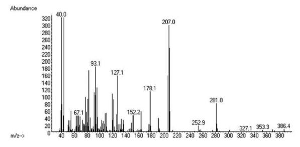
Figure S4. GC-MS (TIC) chromatogram (abscissa: scan number, ordinate: relative response of MS detector) and AMS profile (abscissa: m/z value, ordinate: response of MS detector) of model complex mixture M2.
