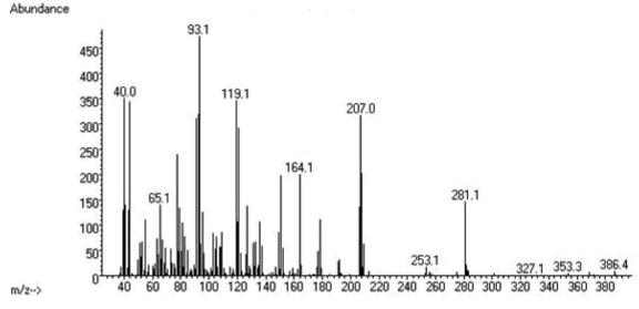
**Figure S5.** GC-MS (TIC) chromatogram (abscissa: scan number, ordinate: relative response of MS detector) and AMS profile (abscissa: m/z value, ordinate: response of MS detector) of model complex mixture M3.
