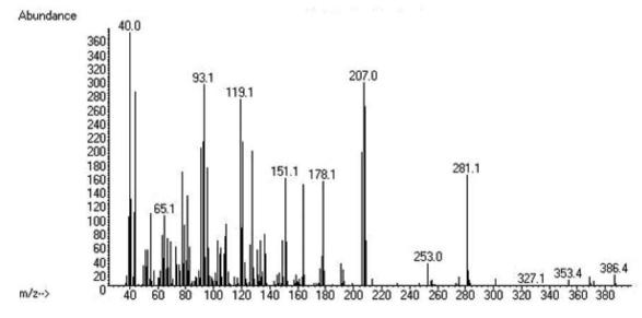
Figure S11. GC-MS (TIC) chromatogram (abscissa: scan number, ordinate: relative response of MS detector) and AMS profile (abscissa: m/z value, ordinate: response of MS detector) of model complex mixture M9.
