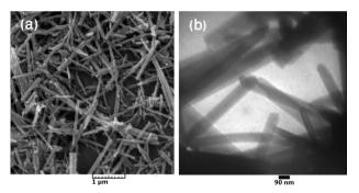
**Figure 6.** (a) SEM and (b) TEM images of the HAp nanorods corresponding to the sample Hy5-200-0.1.
