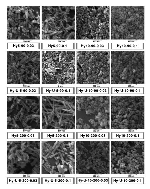
Figure 4. SEM images of the HAp nanoparticles.
