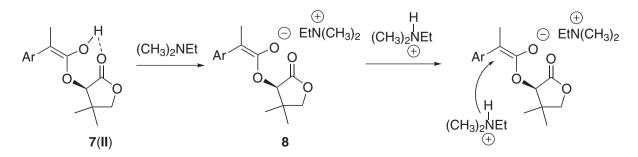
Scheme 5. Mechanism (B): an intermolecular proton transfer, catalyzed by an amine molecule, and an ammonium salt in two successive steps.
