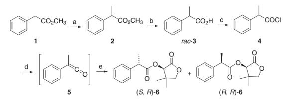
Scheme 1. (a) THF, NaH (0.1 mol), CH<sub>3</sub>I (0.15 mol), reflux, 3 h, 83%; (b) KOH/EtOH, r.t., overnight, 90%; (c) SOCl<sub>2</sub>, reflux, 3 h, 97%; (d) *N*,*N*-dimethylethylamine (1.5 equiv.), 0 °C, 30 min; (e) (*R*)-pantolactone (1.1 equiv., 0.2 mol L<sup>-1</sup> in THF), 0 °C to r.t., 83%, 98% d. e.
