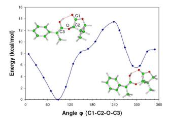
**Figure 1**. Potential curve calculated for the angle ( $\phi$  =C1–C2–O–C3) of the enol identified in Scheme 2 as **7**(**II**).
