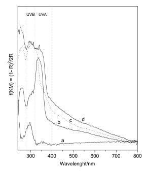
Figure 9. DRUV-VIS spectra of: ZHN (a), sodium *N*-acetylanthranilate (b), *N*-acetylanthranilic acid (c) and ZHN-NAA (d).
