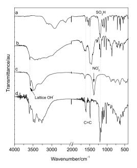
**Figure 3.** FTIR spectra of 4,4'-diamino-2,2'-stilbenedisulfonic acid (a), 4',4-diamino-2,2'-stilbenedisulfonic acid sodium salt (b), ZHN (c) and ZHN-DSD (d).
