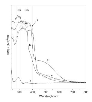
**Figure 4.** DRUV-VIS spectra of ZHN (a), 4,4'-diamino-2,2'stilbenedisulfonic acid (b), 4',4-diamino-2,2'-stilbenedisulfonic sodium salt (c), ZHN-DSD (d) and ZHN-DSD after 2 h stirring in water (e).
