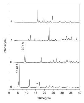
**Figure 2**. XRPD patterns of 4,4'-diamino-2,2'-stilbenedisulfonic acid (a), 4',4-diamino-2,2'-stilbenedisulfonic acid sodium salt (b), ZHN (c) and ZHN-DSD (d).
