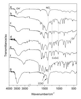
**Figure 8.** FTIR spectra of ZHN (a), sodium methoxycinnamate (b), ZHN-MC (c), sodium methoxybenzoate (d), ZHN-MB (e), sodium *N*-acetylanthranilate (f) and ZHN-NAA (g).
