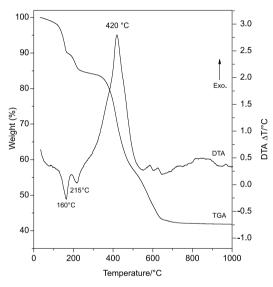
Figure 5. TGA/DTA curves for the ZHN-DSD compound.
