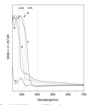
Figure 10. DRUV-VIS spectra of: ZHN (a), sodium 4-methoxycinnamate (b), ZHN-MC (c), sodium 4-methoxybenzoate (d) and ZHN-MB (e).
