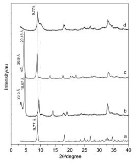
Figure 7. XRPD patterns of ZHN (a), ZHN-MB (b), ZHN-MC (c) and ZHN-NAA (d).
