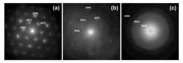
Figure 12. SAED pattern of ZHN obtained at 80 kV and at room temperature (a), ZHN-DSD obtained at 50 kV and at room temperature (b) and ZHN-MC obtained at 50 kV at -43 °C (c). The SAED pattern in (c) was obtained using a cooled specimen holder (Gatan model 636).
