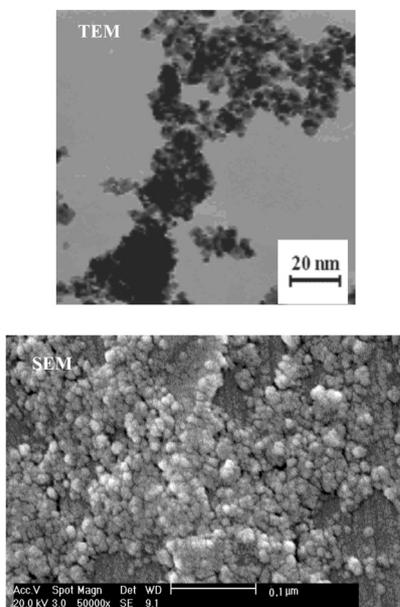
Figure 6. SEM and TEM images registered for the HPA catalyst (× 50000).
