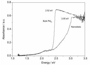
**Figure 2.** Absorption spectra (converted from diffuse reflectance data) of bulk PbI<sub>2</sub> and the CB[7]/PbI<sub>2</sub> sample at 77 K.
