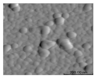
Figure 5. AFM micrograph of the  $CB[7]/PbI_2$  sample with  $CB[7]/PbI_2$  nanoparticle aggregates.
