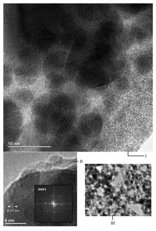
**Figure 6.** HRTEM micrographs of (I) the CB[7]/PbI<sub>2</sub> sample; (II) a single PbI<sub>2</sub> nanodisk (diameter *ca.* 30 nm), inset: electron diffraction pattern; and (III) CB[7]/PbI<sub>2</sub> sample under higher magnification, with random nanodisks in a "house of cards" arrangement.
