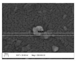
Figure 4. SEM image of the CB[7]/PbI<sub>2</sub> sample with aggregates under  $\times$  200,000 magnification. The grain size estimated in 54 nm.
