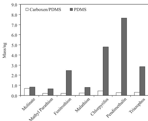
**Figure 1.** Extracted amount for the pesticides obtained with two different thicknesses of the polydimethylsiloxane fiber. Experimental conditions: 100  $\mu\text{m}$  PDMS and 75  $\mu\text{m}$  carboxen-PDMS fibers, 30 min extraction; sample volume, 30 mL; stirring (150 rpm), Milli-Q water at pH 7 and spiked with 4  $\mu\text{g L}^{-1}$  of each analyte.
