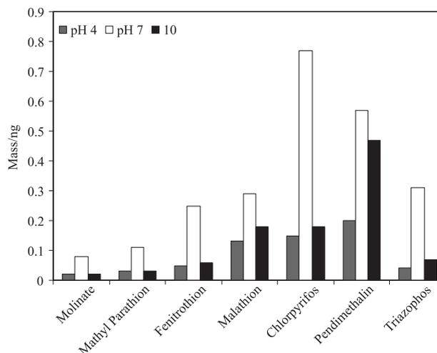
**Figure 2.** Influence of pH of the sample. Experimental conditions:  $100 \mu\text{m}$  PDMS, 30 min extraction; sample volume 30 mL; stirring (150 rpm) and  $1 \mu\text{g L}^{-1}$  of each analyte.
