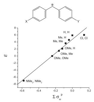
**Figure 6.** Plot of the electrophilicity *E* of diarylcarbenium ions ArAr'CH<sup>+</sup> vs. the sum of the corresponding  $\sigma_0^{p}$  values (correlation  $R^2 = 0.97$ ). The electrophilicities *E* were obtained from reference 18.
