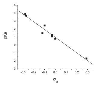
**Figure 4.** Plot of pKa values of protonated pyridine N-oxides *vs.* the corresponding substituent electrophilic  $\sigma_{\omega}$  values (correlation R<sup>2</sup> = 0.96). pKa values were obtained from reference 14 and 15.
