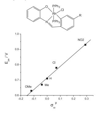
**Figure 7.** Plot of the oxidation potential of Rh(III) to Rh(IV) in a substituted benzaldimine complex *vs.* the electrophilic  $\sigma_{\omega}^{p}$  value of substituents R (correlation R<sup>2</sup> = 0.99). Experimental data were obtained from reference 20.
