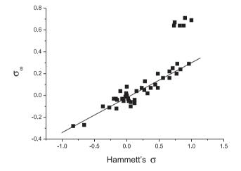
**Figure 8.** Plot of electrophilic  $\sigma_{\omega}$  vs. Hammett's  $\sigma$  constants for all *meta-* and *para-*substituents of Table 1 (correlation R<sup>2</sup> = 0.88). The points above the straight line correspond to positively charged substituents (Me<sub>3</sub>N<sup>+</sup>, Me<sub>2</sub>P<sup>+</sup>, Me<sub>2</sub>S<sup>+</sup>)
