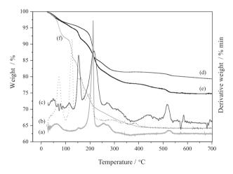
**Figure 3.** DTG curves of (a) LHS-Pd<sup>0</sup>, (b) zinc hydroxide acetate (LHS) and (c) LHS60 and TG curves of (d) LHS-Pd<sup>0</sup>, (e) LHS60 and (f) zinc hydroxide acetate (LHS).
