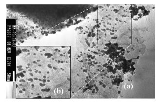
Figure 2. TEM images of (a) LHS-Pd<sup>0</sup> and (b) zoom of the marked area in (a).
