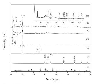
**Figure 1.** XRD patterns of (a)  $K_2PdCl_6$ , (b) ZnO, (c) Zn(OAc)<sub>2</sub>, (d) zinc hydroxide acetate (LHS), (e) LHS60, (f) LHS-Pd<sup>0</sup> and (g) characteristic peaks for Pd<sup>0</sup> in LHS-Pd<sup>0</sup>.
