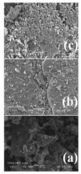
Figure 4. SEM images of (a) zinc hydroxide acetate (LHS), (b) LHS60 and (c) LHS-Pd $^{0}$ .
