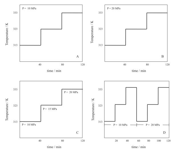
**Figure 1.** Extraction step design, A: three steps (313, 323, 333 K) each one at 10 MPa for 40 min, B: three steps (313, 323, 333 K) each one at 20 MPa for 40 min, C: three steps (313/10, 323/15, 333/20 K/MPa) each one for 40 min, D: six steps (313/10, 323/10, 313/20, 323/20, 333/20 K/MPa) each one for 20 min.
