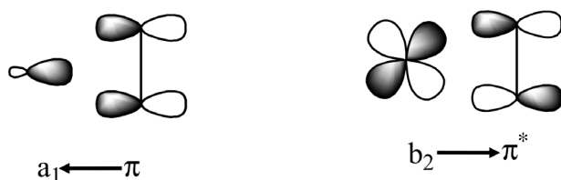
Scheme 1. Ligand \sigma donation to metal ( a_1 \leftarrow \pi ) and metal to ligand \pi back-donation ( b_2 \rightarrow \pi^* ), according to the orbital interactions in the Dewar-Chatt-Duncanson model.
