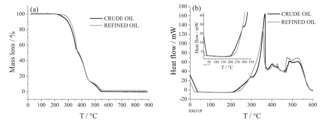
Figure 2. Thermogravimetric (a) and calorimetric curves (b) for crude and refined buriti oil samples.
