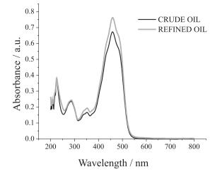
Figure 1. Absorption spectra of buriti oils in UV-Vis.
