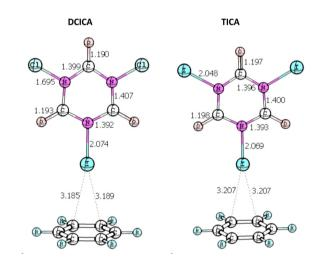
**Figure 5.**  $\pi$ -Complexes between benzene and DCICA and TICA obtained at M06-2X/6-311++G(d,p) level.
