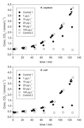
**Figure 2.** Bacterial growth of *K. oxytoca* and *E. coli* in the presence of  $Hg^{2+}$ .
