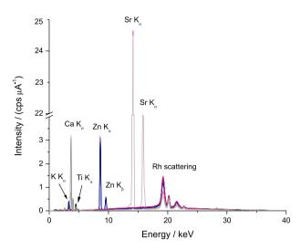
Figure 2. Direct X-ray spectra of 16 toothpaste samples of the PLS calibration set.
