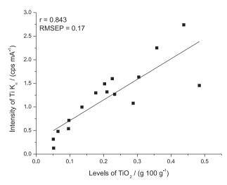
**Figure 5.** Intensity of Ti K<sub> $\alpha$ </sub> peak *vs.* Ti concentration, after direct irradiation of 16 toothpaste samples (univariate calibration).
