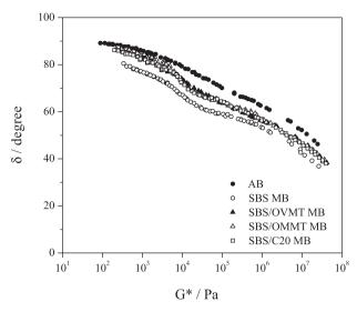
Figure 5. Black diagrams for pure asphalt binder and modified binders.
