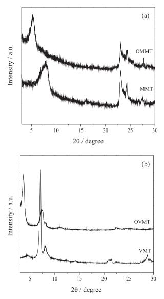
**Figure 1.** X-ray diffractograms for (a) OMMT and MMT and (b) OVMT and VMT.
