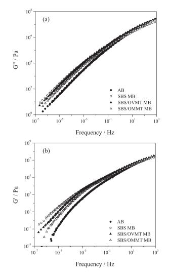
**Figure 3.** Master curves for (a) viscous modulus (G') and (b) elastic modulus (G') for pure asphalt binder and modified binders as a function of frequency at a reference temperature of 25 °C.
