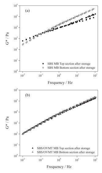
**Figure 6**. G\* as a function of frequency for (a) SBS MB and (b) SBS/OVMT MB after storage at a temperature of 60  $^{\circ}$ C.
