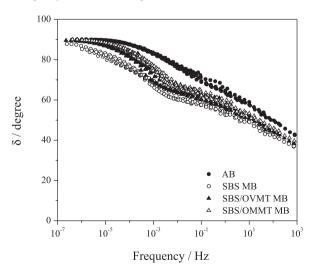
Figure 4. Master curves of phase angle ( $\delta$ ) for pure asphalt binder and modified binders as a function of frequency at a reference temperature of 25 °C.
