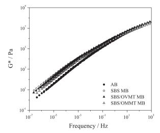
**Figure 2**. Master curves of complex modulus ( $G^*$ ) for pure asphalt binder and modified binders as a function of frequency at a reference temperature of 25 °C.
