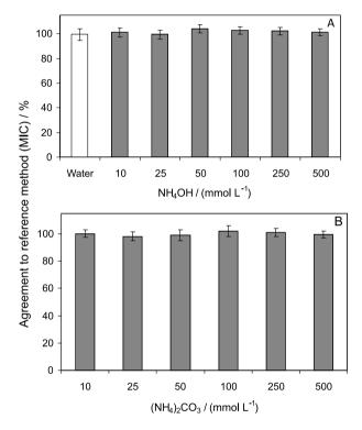
Figure 1. Agreement obtained for F after pyrohydrolysis of CNT using (A) water (vapor condensed during pyrohydrolysis reaction) and ammonium hydroxide and (B) ammonium carbonate as absorbing solutions (results were compared with values obtained after MIC digestion). Error bars correspond to standard deviation (n = 3). Pyrohydrolysis conditions: 500 mg of sample, temperature of 950 °C, 10 min of reaction and air flow rate of 200 mL min<sup>-1</sup>.
