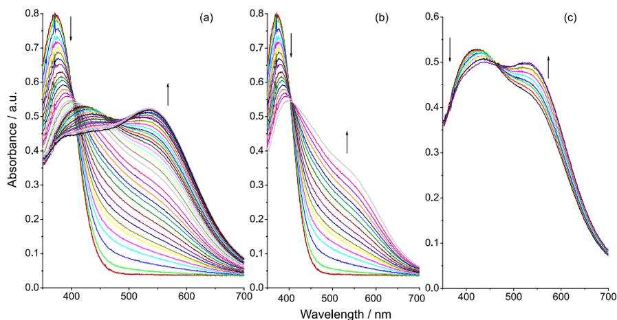
**Figure 5.** (a) Influence of the addition of increasing amounts of  $\text{F}^-$  on the UV-Vis spectra of **2a** ( $5.0 \times 10^{-5} \text{ mol L}^{-1}$ ) in acetonitrile at 25 °C. The final concentration of  $\text{F}^-$  was  $9.02 \times 10^{-4} \text{ mol L}^{-1}$ ; (b) the first step of this titration from zero to  $1.85 \times 10^{-4} \text{ mol L}^{-1}$  and (c) the last step from  $3.58 \times 10^{-4} \text{ mol L}^{-1}$  to  $6.11 \times 10^{-4} \text{ mol L}^{-1}$ .
