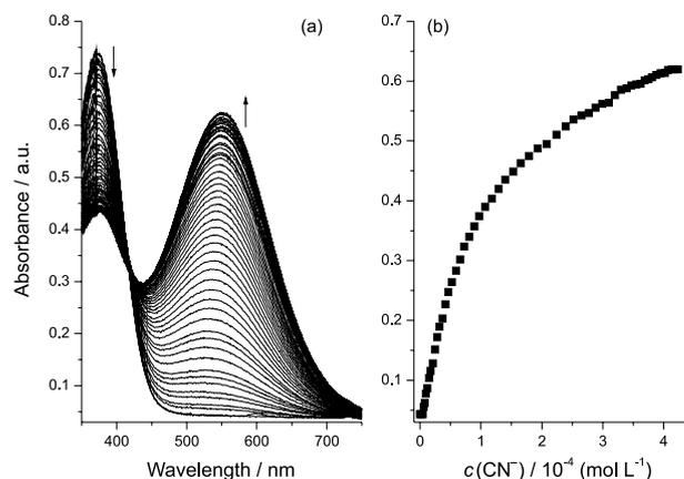
**Figure 3.** (a) Influence of the addition of increasing amounts of CN<sup>-</sup> on the UV-Vis spectra of **2a** ( $5.0 \times 10^{-5}$  mol L<sup>-1</sup>) in acetonitrile at 25 °C. The final concentration of CN<sup>-</sup> was  $4.18 \times 10^{-4}$  mol L<sup>-1</sup>; (b) curve of the variation in the absorbance at 547.0 nm of **2a** with the addition of increasing amounts of CN<sup>-</sup>.
