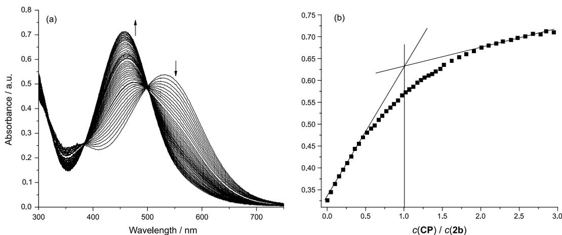
**Figure 6.** (a) UV-Vis spectra of **2b** ( $4.0 \times 10^{-5} \text{ mol L}^{-1}$ ) in acetonitrile at 25 °C after addition of increasing amounts of **CP**. The final concentration of **CP** was  $1.2 \times 10^{-4} \text{ mol L}^{-1}$ ; (b) mole-ratio plot for the interaction of **CP** with **2b**.
