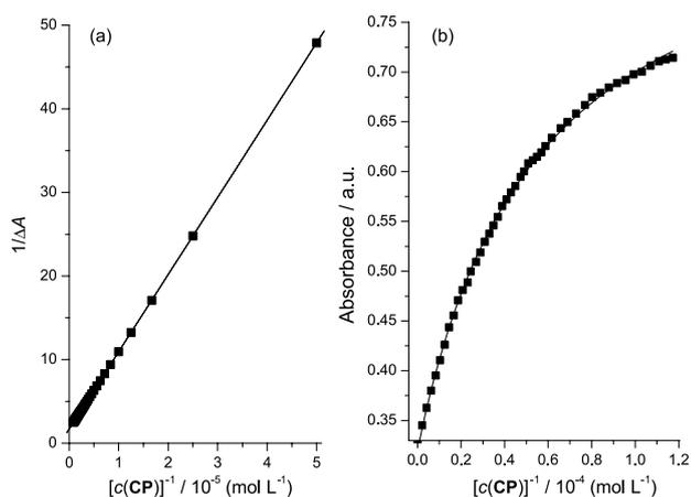
**Figure 7.** (a) Benesi-Hildebrand treatment for the titration of  $\mathbf{2b}$  and  $\mathbf{CP}$  in acetonitrile at 25 °C, fitted using equation 3; (b) titration curve of  $\mathbf{2b}$  and  $\mathbf{CP}$  in acetonitrile at 25 °C. Absorbance values were collected at 456.0 nm and the data were fitted using equation 2.
