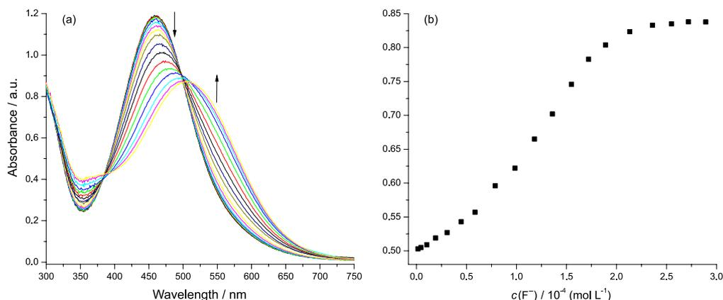
**Figure 9.** (a) UV-Vis spectra of **CP-2b** in acetonitrile at 25 °C after addition of increasing amounts of  $\text{F}^-$ ; (b) titration curve of **CP-2b** with  $\text{F}^-$  in acetonitrile. Absorbance values were collected at 547.0 nm,  $c(\text{CP}) = 1.2 \times 10^{-4} \text{ mol L}^{-1}$  and  $c(\text{2b}) = 4.0 \times 10^{-5} \text{ mol L}^{-1}$ .
