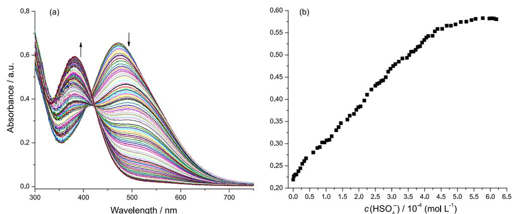
**Figure 10.** (a) UV-Vis spectra of **CP-2b** in acetonitrile at 25 °C after addition of increasing amounts of  $\text{HSO}_4^-$ ; (b) titration curve of **CP-2b** with  $\text{HSO}_4^-$  in acetonitrile. Absorbance values were collected at 372.0 nm,  $c(\text{CP}) = 1.2 \times 10^{-4} \text{ mol L}^{-1}$  and  $c(\text{2b}) = 4.0 \times 10^{-5} \text{ mol L}^{-1}$ .
