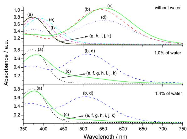
**Figure 2.** UV-Vis spectra for solutions of (a) **2a**, (b) **2b** and **2a** in the presence of (c)  $\text{F}^-$ , (d)  $\text{CN}^-$ , (e)  $\text{CH}_3\text{COO}^-$  and (f)  $\text{H}_2\text{PO}_4^-$  in acetonitrile and acetonitrile with 1.0 and 1.4% (v/v) of water. For concentrations of **2a** and the anions, see Figure 1.
