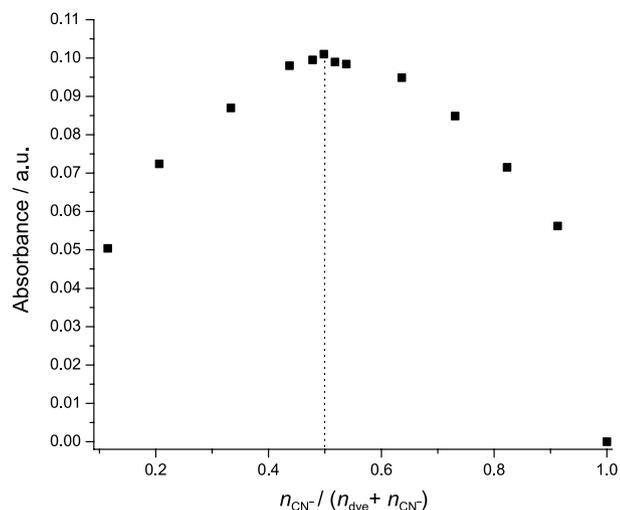
**Figure 4.** Job plot of **2a** with  $\text{CN}^-$  in acetonitrile (for details see Experimental section).
