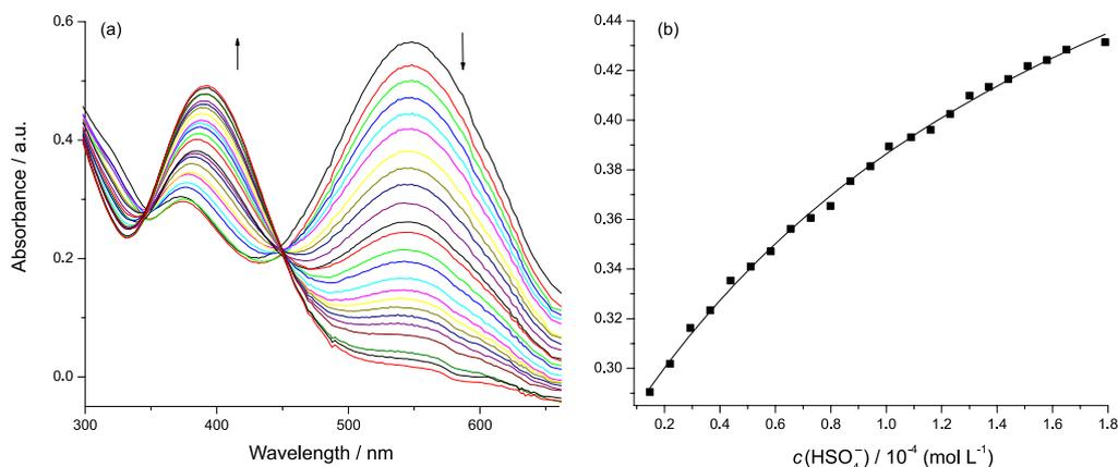
**Figure 11.** (a) UV-Vis spectra of **2b** ( $4.0 \times 10^{-5} \text{ mol L}^{-1}$ ) in acetonitrile at  $25 \text{ }^\circ\text{C}$  after addition of increasing amounts of  $\text{HSO}_4^-$ ; (b) titration curve of **2b** with  $\text{HSO}_4^-$  in acetonitrile, with the absorbance values collected at  $372.0 \text{ nm}$ .
