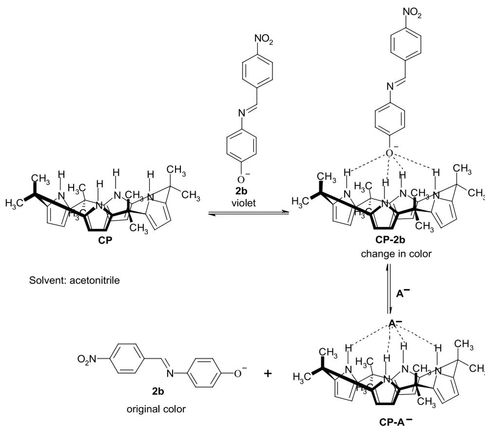
**Scheme 3.** A chromogenic chemosensor based on a displacement assay.
