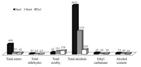
Figure 1. Median concentration (mg  $L^{-1}$ ) of secondary composition, ethyl carbamate ( $\mu$ g  $L^{-1}$ ) and alcoholic content (%, v/v) in the three fractions produced in alembic distillation.
