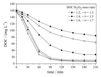
Figure 2. DOC concentration variation over time for degradation by  $UV/H_2O_2$  at different DOC: $H_2O_2$  mass ratios.
