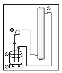
**Figure 1.** Experiment setup: (1) magnetic stirrer, (2) vessel, (3) peristaltic pump and (4) photochemical reactor.
