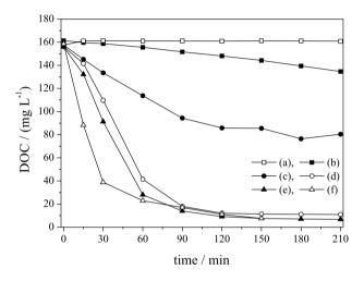
**Figure 5.** DOC value variation over time during treatment by (a)  $H_2O_2$  (DOC: $H_2O_2$  1:7 mass ratio), (b) UV, (c) Fenton's reagent (250 mg L<sup>-1</sup> Fe(II) and DOC: $H_2O_2$  1:7 mass ratio), (d) UV/ $H_2O_2$  (DOC: $H_2O_2$  1:5 mass ratio), (e) UV/ $H_2O_2$  (DOC: $H_2O_2$  1:7 mass ratio) and (f) photo-Fenton (31 mg L<sup>-1</sup> Fe(II) and DOC: $H_2O_2$  1:5 mass ratio).
