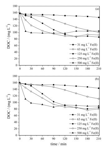
Figure 3. DOC values at different Fe(II) concentrations over time for (a) 1:5 and (b) 1:7 DOC: $H_2O_2$  mass ratios, for the Fenton process.
