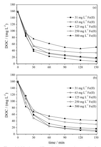
**Figure 4.** DOC values at different Fe(II) concentrations over time for (a) 1:5 and (b) 1:7 DOC: $H_2O_2$  mass ratios for the photo-Fenton process.
