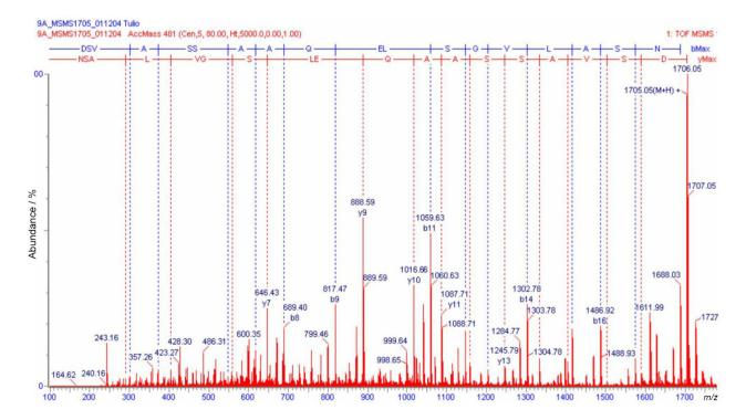
Figure 1. De novo sequencing of the peptide otacidin (O. taurinus) m/z 1706.05 [M + H]<sup>+</sup>. An Applied 4700 Proteomics mass spectrometer was used with N<sub>2</sub> as CID gas. The observed fragments allowed complete assignment of the major y- and b- ion series. The peptide sequence using one-letter code following the y- and b- series orientation is shown on the top part of the graph.
