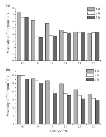
Figure 3. Viscosity of (a) BB and (b) COB.
