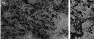
Figure 2. SEM of (a) SrCO<sub>3</sub> and (b) SrCO<sub>3</sub> + SrO + Sr(OH)<sub>2</sub>]
