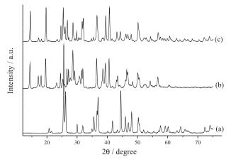
**Figure 1.** Diffratograms of (a)  $SrCO_3$ , (b)  $[SrCO_3 + SrO + Sr(OH)_2]$  and (c)  $SrO.xH_2O$ .
