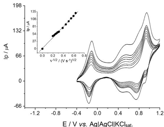
**Figure 5.** Cyclic voltammograms obtained at a glassy carbon electrode modified with a thin film of ruthenium-based hexacyanoferrate in Britton-Robinson buffer solution at pH 1.5 in the presence of 0.1 mol L<sup>-1</sup> ethanol at different scan rates (0.04, 0.05, 0.06, 0.07, 0.08, 0.09, 0.1 and 0.15 V s<sup>-1</sup>). Inset figure: plot of  $I_{pa}$  vs.  $v^{1/2}$ .
