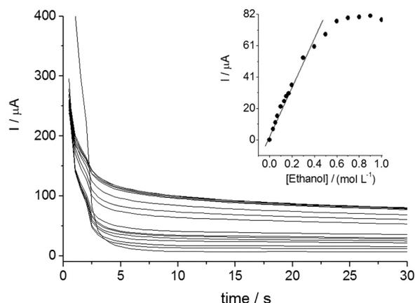
**Figure 8.** Chronoamperometric responses of the glassy carbon electrode modified with a mixed film of ruthenium-based hexacyanoferrate in Britton-Robinson buffer solution at pH 1.5 at different ethanol concentrations. Inset figure: Plot of  $I_a$  vs. [ethanol].
