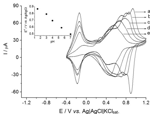
**Figure 3.** Cyclic voltammograms obtained at a glassy carbon electrode modified with a mixed film of ruthenium-based hexacyanoferrate at different pH values of 0.1 mol L<sup>-1</sup> Britton-Robinson buffer solution: (a) 1.5, (b) 3.0, (c) 4.0, (d) 5.5 and (e) 7.0,  $v = 0.1$  V s<sup>-1</sup>. Inset figure: plot of  $E^{\circ}$  vs. pH.
