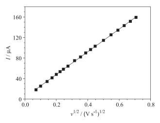
**Figure 6.** Linear dependence of the peak current  $(I_{ap})$  with the square root of the scan rate  $(\nu^{1/2})$  for cyclic voltammograms of a 1.0 mmol L<sup>-1</sup> PTU solution in the BR buffer (pH 2.0) using a cathodically BDD electrode at different scan rates (0.005-0.500 V s<sup>-1</sup>).
