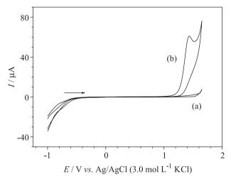
**Figure 2.** Cyclic voltammograms (50 mV s<sup>-1</sup>) obtained using a cathodically pretreated BDD electrode for a: (a) BR buffer solution (pH 2.0); (b) 1.0 mmol L<sup>-1</sup> PTU solution in the BR buffer (pH 2.0).
