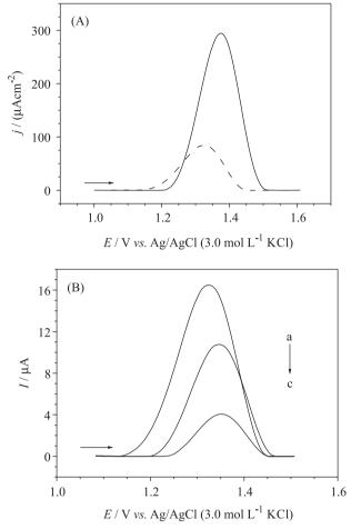
**Figure 8.** Differential pulse voltammograms for a 500  $\mu$ mol L<sup>-1</sup> PTU solution in the BR buffer (pH 2.0) obtained on: (A) GC (dashed line) and BDD (solid line) electrodes; (B) a GC electrode for the (a) first, (b) second, and (c) third scans.
