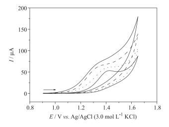
**Figure 5.** Cyclic voltammograms (50 mV s<sup>-1</sup>) of 1.0 mmol L<sup>-1</sup> PTU solutions in BR buffers of different pH values: 2.0 (solid thick line), 3.0 (dotted line), 4.0 (dashed line), and 5.0 (solid line) using a cathodically pretreated BDD electrode.
