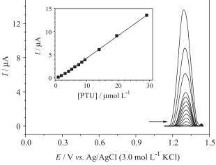
Figure 7. Differential pulse voltammograms obtained using the cathodically pretreated BDD electrode for (1) 1.0, (2) 2.0, (3) 3.2, (4) 4.3, (5) 5.3, (6) 6.3, (7) 7.5, (8) 8.5, (9) 9.5, (10) 14.0, (11) 20.0, and (12) 29.1 µmol L<sup>-1</sup> PTU solutions in the BR buffer (pH 2.0). Insert: corresponding analytical curve.
