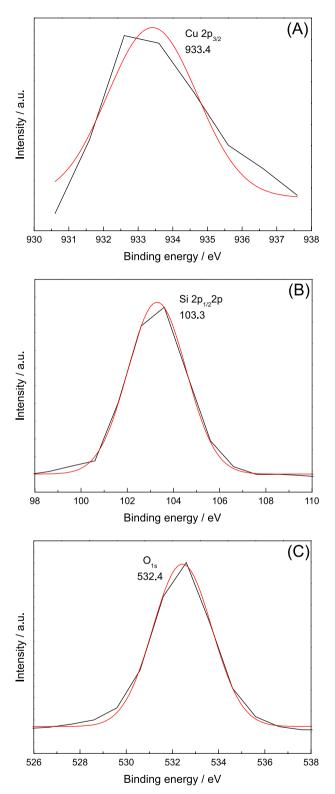
**Figure 5**. XPS spectra of the catalysts  $SiO_{2(1-x)}Cu_x$ : (A) region Cu  $2p_{3/2}$ ; (B) region Si  $2p_{1/2}2p$  and (C) region  $O_{1s}$ .
