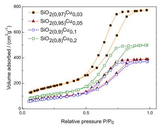
Figure 1. Nitrogen isotherms of the catalysts SiO<sub>2(1-x)</sub>Cu<sub>x</sub>.
