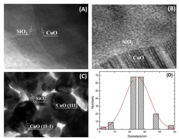
Figure 4. TEM images of (A)  $SiO_{2(0.95)}Cu_{0.05}$ ; (B)  $SiO_{2(0.8)}Cu_{0.2}$ ; (C)  $SiO_{2(0.9)}Cu_{0.1}$  and (D) particle size distribution for copper of  $SiO_{2(0.9)}Cu_{0.1}$ .
