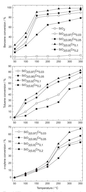
**Figure 6**. BTX conversion as a function of reaction temperature for different catalysts under varying reaction conditions: benzene 2.0 g  $m^3$ , toluene 0.5 g  $m^3$ , o-xylene 0.4 g  $m^3$ . Total flow rate: 20 ml min<sup>-1</sup>.
