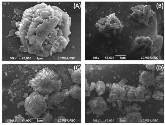
Figure 3. SEM images of (A)  $SiO_{2(0.97)}Cu_{0.03}$ ; (B)  $SiO_{2(0.95)}Cu_{0.05}$ ; (C)  $SiO_{2(0.9)}Cu_{0.1}$  and (D)  $SiO_{2(0.8)}Cu_{0.2}$ .
