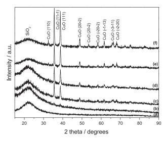
Figure 2. XRD patterns for the samples (a) SiO<sub>2</sub>; (b) SiO<sub>2(0.97)</sub>Cu<sub>0.03</sub>; (c) SiO<sub>2(0.95)</sub>Cu<sub>0.05</sub>; (d) SiO<sub>2(0.9)</sub>Cu<sub>0.1</sub> and (e) SiO<sub>2(0.8)</sub>Cu<sub>0.2</sub>.
