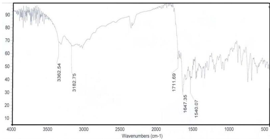
Figure S4. IR spectrum of compound 3.
