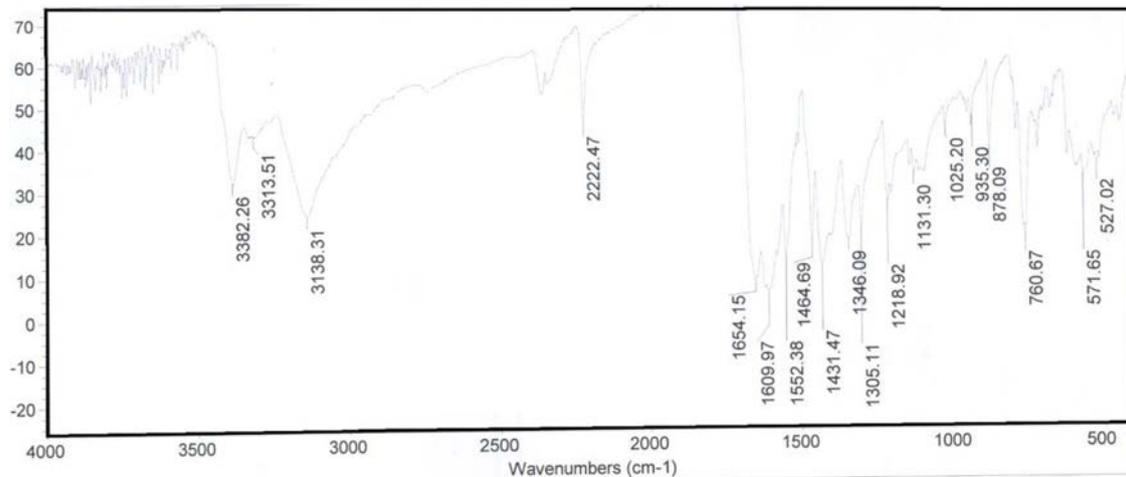
Figure S38. IR spectrum of compound **19**.
