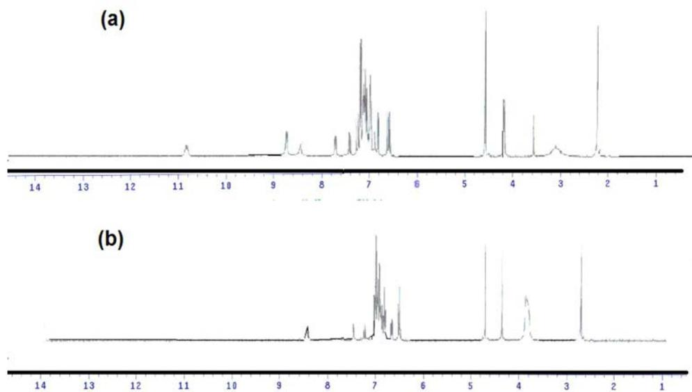
Figure S5. <sup>1</sup>H NMR spectra of compound 3 in DMSO-*d*<sub>6</sub> (a) and DMSO-D<sub>2</sub>O (b).
