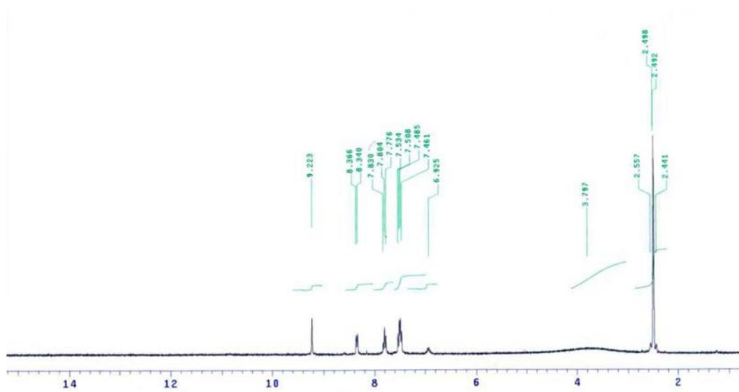
Figure S22. <sup>1</sup>H NMR spectrum of compound 12 in DMSO-*d*<sub>6</sub>.
