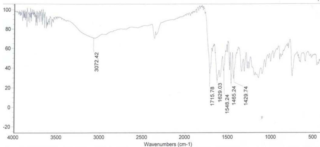
Figure S31. IR spectrum of compound 15.
