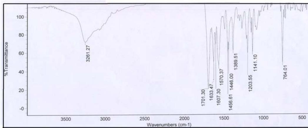
Figure S25. IR spectrum of compound 13.
